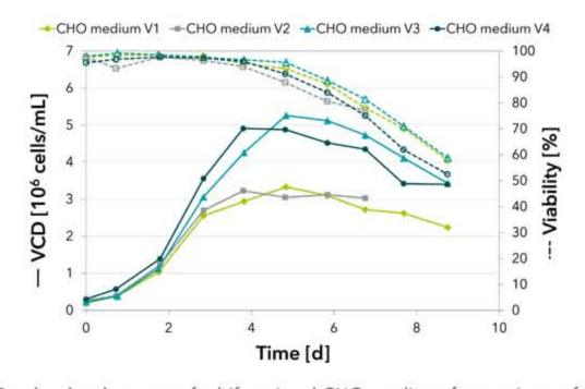
For the development of a bifunctional CHO medium, four variants of medium A and B were further tested and optimized with regard to cell growth. A batch curve of transient CHO cell line 3 in these early stage variants of CHO medium B is shown.
