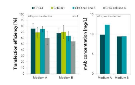
Transfection efficiencies measured in two early development stages of CHO medium A and B 48 h post transfection (n ≥ 4 independent experiments). Additionally, for two CHO cell lines, the expression of a monoclonal antibody was measured 48 h post transfection. The cultivation before and after transfection was performed in reference growth medium.
